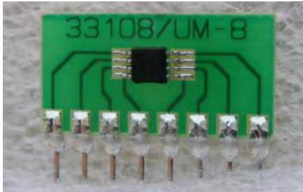
Fig.1. Surface-mount adaptors are available from all the distributors, but are disproportionately expensive.
